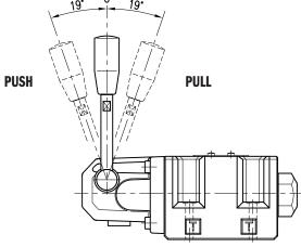
On 3- position valves, pulling the lever obtains the right position, pushing the lever obtains the left position  $\,$
