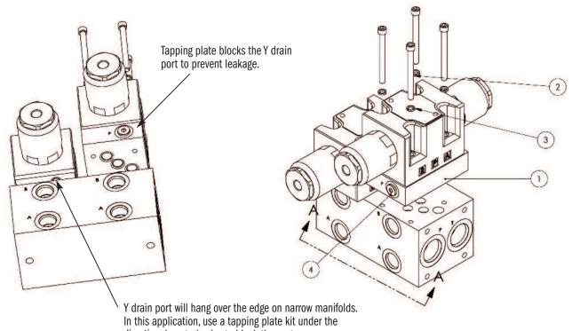
In this application, use a tapping plate kit under the directional control valve to block the port.
