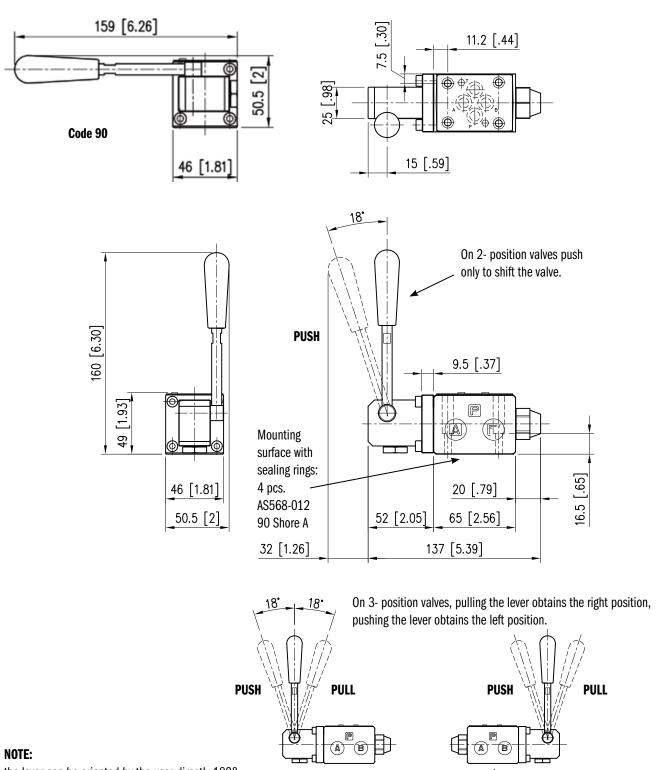
the lever can be oriented by the user directly  $180^{\circ}$  turned to the standard position by uscrewing the lever and re-mounting it in the desired position.
