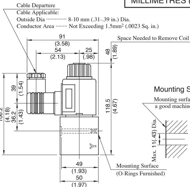
Note 1: For models with DC solenoids and models with R type solenoids, refer to CDST-03, 03W.
