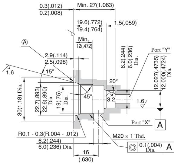
Note: The fitting portion of o-rings should have a good machined finish.
