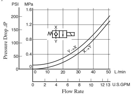
Note: Measuring has been made for the CDSC-03 (Cartridge type) when it is equipped with the same body as the threaded connections and the gasket mounting type.
