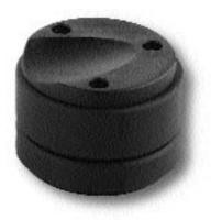
The SWR is a compact switched rocker offering finger tip/thumb control in up to 4 half axes. The unit is supplied with an 'O' ring so as to ensure IP66 sealing above the panel and is capable of switching a resistive load of up to 100mA.
